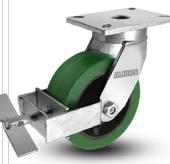
Available on all swivel and rigid casters, except stainless and spring loaded. Turn lever to apply shoe against wheel tread for positive locking action. Add **F** to end of part number for factory orders.
