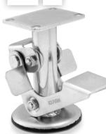
The Albion 02 Series floor locks are designed to hold your portable equipment in a desired location. Intended for use on level surfaces, the floor lock is activated by toe pressure on the extension pedal or released by toe touching one of the dual retractable plates. For best results, units should be used in pairs.
