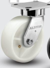
The 120 Series is constructed from 304 stainless steel and features a precision machined swivel section that is welded inside and outside to legs for maximum durability. The stainless construction is highly polished and ideal for applications exposed to cleaning agents, washdowns, caustic solutions, steam, marine environments or any other corrosive agents that could cause rust.
