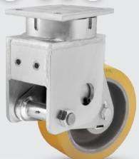
Designed from high quality, heat treated AISI 1045 stamped steel. Zinc plating delivers greater corrosion resistance than paint. Inside and outside welds deliver superior strength.
