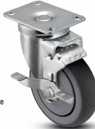
**Example model number** shown (PGS50120ZN-TPR33(GG) TB) is an institutional caster (**PGS**). The wheel diameter is 5" (**50**). The fastening is a swivel top plate (**120**). The caster fork finish is zinc (**ZN**). The wheel is a TPR (**TPR**) with a precision bearing and full thread guard (**33**). The color of the tread is grey and the wheel core is grey (**GG**). The caster has an optional tread lock brake (**TB**).
