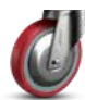
Hi-Temp Thermal Rubber (ARZ) 280 degrees Wash down (10 minutes), Auto Clave / Steam Sterilizer instrument wash @ max load of 200lb per wheel under heat and 250lb at room temp. Durometer: 70A±5
