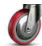
Hi-Temp Thermal Rubber (ARZ) 280 degrees Wash down (10 minutes), Auto Clave / Steam Sterilizer instrument wash @ max load of 200lb per wheel under heat and 250lb at room temp. Durometer: 70A±5
