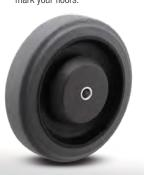
SuperKat wheels feature a soft natural rubber tread material along with a more rounded tread shape. This design allows the wheel to rotate as it is pulled sideways by cart pusher machines. Because the wheel is allowed to spin, even with sharp turns, it is much more resistant to flat spotting compared to conventional wheels. This design has been used successfully in Europe for over 20 years.
